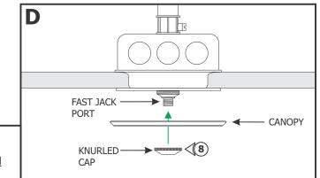
8: Place the canopy onto the Fast Jack port assembly against the electrical box and secure it in place by tightening the knurled cap to the Fast Jack port. <u>Make sure the knurled</u> <u>cap is not cross threaded.</u>
