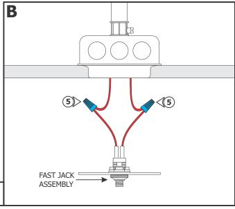
**5:** Connect each Fast Jack assembly wire to one low voltage transformer wire with a wire nut.
